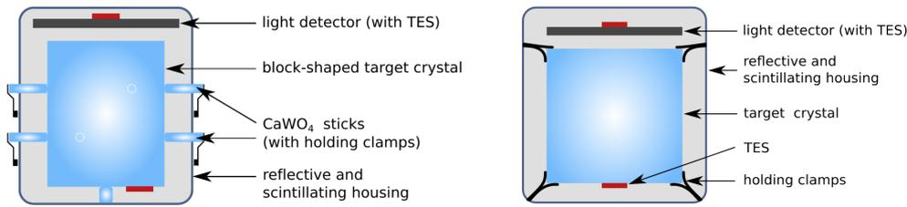
Figure 1: Schematic drawings of the setup of the detector modules TUM40 (left) and Lise (right).
